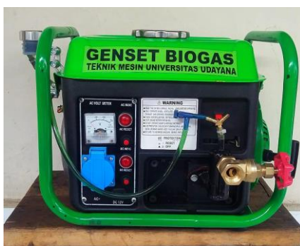
Fig. 1. Familiar 2 stroke single cylinder (63 cc) engine of 750 watt electric generator. This small electric generator was set to be fuelled with biogas.
