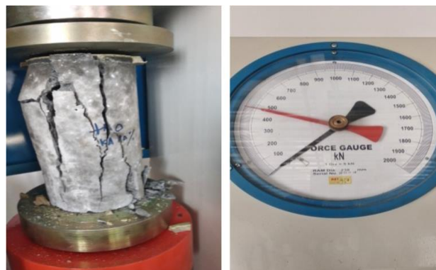
Figure 1. Compressive Test Of Concrete
